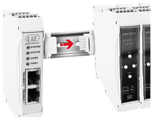
Fig. 4.6: Connection of an MSC7602 with MSC7602 connector set
